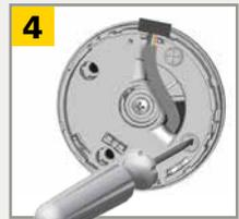
Position the bracket and fasten the 4 screws firmly.
