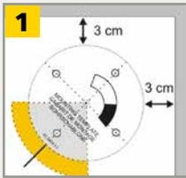
Use the adhesive mounting template to position the sensor correctly. The grey area indicates the detection range.
