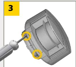
3 **Lock the position** of the mounting bracket to avoid malfunctioning in case of extreme vibrations.
