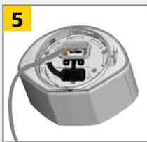
Open the protection cover, plug the connector and position the cable in the slit.
