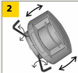
2 Adjust the **tilt angle** of the detection field with the hex key.
