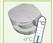
Keep the sensor permanently powered in environments where the temperature can descend below 0°C.
