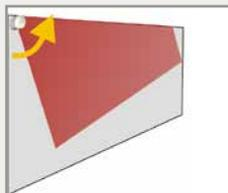
The sensor memorizes the floor as reference point and will signal a fault in case the orientation of the sensor is changed (on purpose or by accident).
