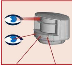
Do not look into the laser emitter or the visible red laser beams.
