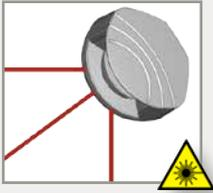
The visible laser beams indicate approximately the position of curtain C1 and limit the angle of the detection field.
