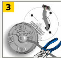
Pass the cable +/- 10 cm through the cable opening. If drilling an opening is not possible, use the cable conduits on the back side of the bracket.
