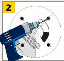
Drill 4 holes as indicated on the mounting template. Make a hole for the cable if possible.
