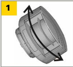
1 Adjust the **lateral position** of the detection field.
