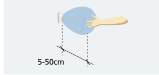
**Flexible short-range detection filed** User defined detection range from 5 to 50 cm.
