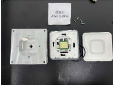
IP6X After test
