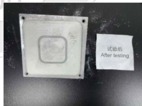
IP6X After test
