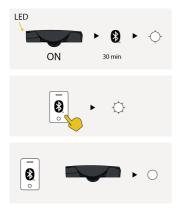
At power ON or after a power cycle, the Bluetooth® is activated for 30 min and the Bluetooth® LED is flashing white.
